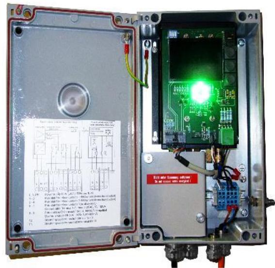
Figure 3: Configuration of EKV-4 in gas hazardous areas with opened enclosure and power switched on
