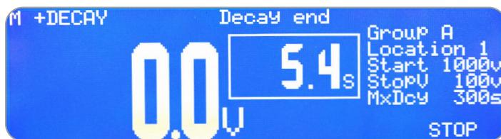
The Model 280A CPM displays an easy to view LCD screen for tracking of your operating parameters. Users can set the test parameters all by the simple push of a button.
