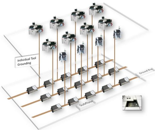
Filtering Ground in Subfloor
