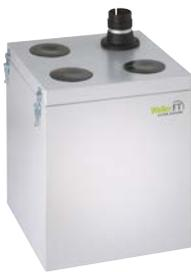
The Pre-filter is recommended for use with solder bath, automatic soldering, laser or other major dust emitting applications. It acts as a first stage in the filter process increasing the lifetime of the main filter units. The Pre-filter can be fixed directly to the top of the ZS 6V or in conjunction with all Weller FT volume extraction units as an external part of the fume extraction system.
