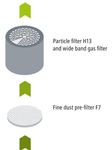
Particle filter H13 and wide band gas filter
