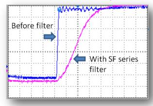
Bearings' Ground Current Reduced 50...100 Times
