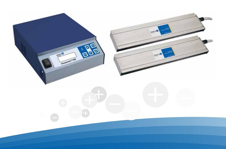
Chargemaster systems utilize high frequency switching technology, which offers three major advantages. First, it ensures that the voltage output from the power supply is equal to the voltage requested via the controls. Second, fluctuations on the AC input line will not affect the voltage output. Finally, variances in load, up to the recommended maximum, do not affect the voltage output.
